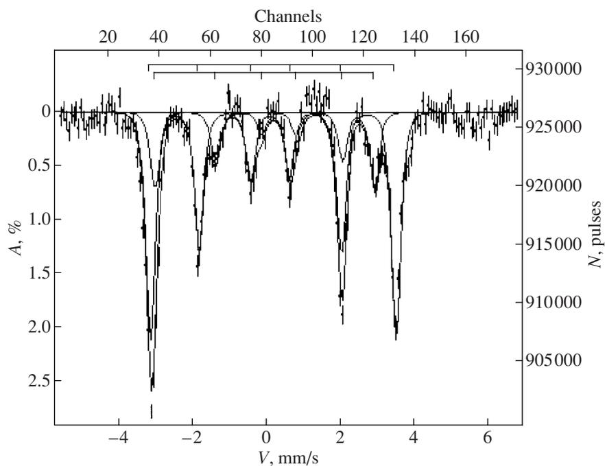
Fig. 5. Mössbauer spectrum of the  $\text{Tb}_{0.3}\text{Dy}_{0.7}\text{Fe}_2$  alloy.
