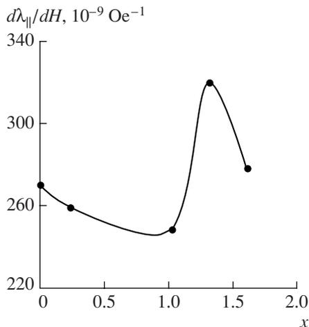
Fig. 4. Concentration dependence of  $\partial\lambda_{||}/\partial H$  for the  $\text{Tb}_{0.3}\text{Ho}_{0.03}\text{Dy}_{0.67}\text{Fe}_{2-x}\text{Co}_x$  system alloys at  $T = 300$  K.
