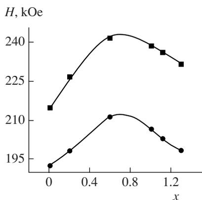
Fig. 6. Superfine field in the  $\text{Tb}_{0.3}\text{Dy}_{0.7}\text{Fe}_2$  alloy as a function of  $x$ .
