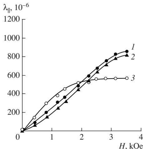
Fig. 3. Field dependence of longitudinal magnetostriction  $\lambda$  for the  $\text{Tb}_{0.3}\text{Dy}_{0.7}\text{Fe}_{2-x}\text{Co}_x$  compounds at  $x = (1) 0, (2) 0.2,$  and  $(3) 1.3$  at  $T = 300$  K.
