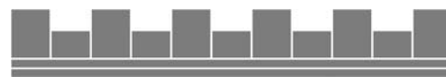
Fig. 5. Longitudinal section of a three-layer axially symmetric structure of piecewise constant radius, assuming two values for 11 sections.
