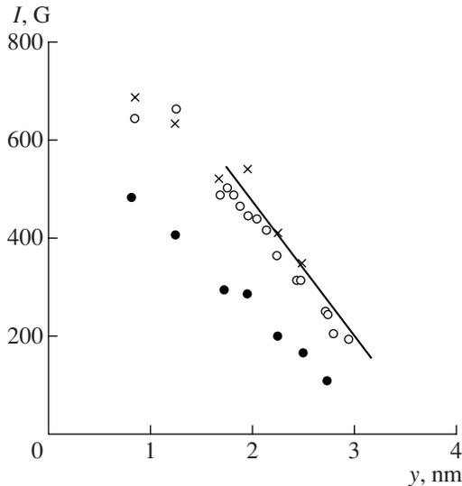
**Fig. 4.** Dependences of the magnetization on  $y$  in samples of series 1.  $\times$ ,  $I_{\text{weak}}$ ;  $\bullet$ ,  $I_m$ ;  $\circ$ ,  $I$  from the FMR data; solid line, calculated according to Eq. (2).
