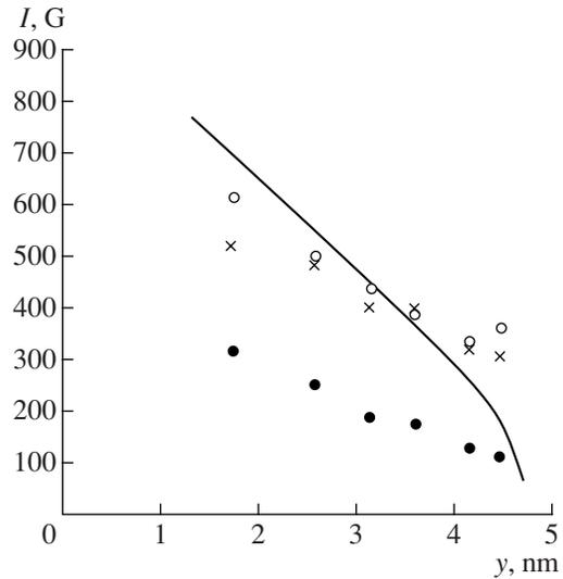
**Fig. 5.** Dependences of the magnetization on  $y$  in samples of series 2. Notations are the same as in Fig. 4.
