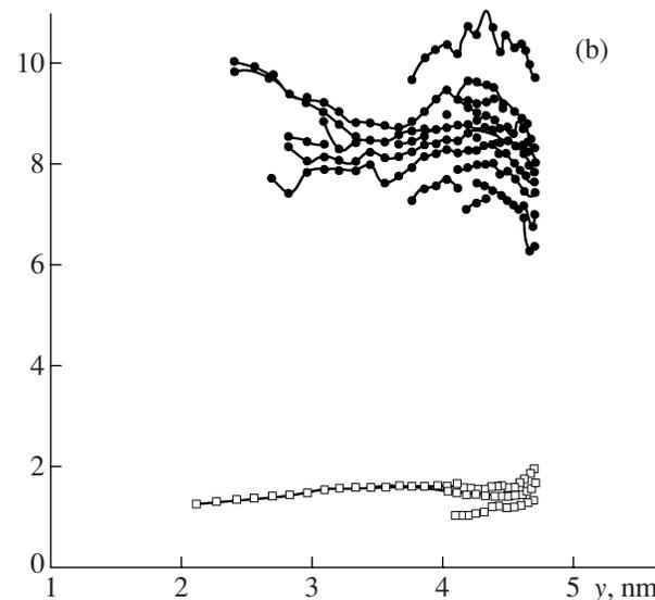
**Fig. 3.** Dependences of the resonance fields of different lines in the magnetostatic vibration spectrum on the interlayer thickness ( $y$ ).  $\bullet$ ,  $\mathbf{H}_{\perp}$ ;  $\square$ ,  $\mathbf{H}_{\parallel}$ . Solid lines connect resonances of supposedly similar vibration types. Bold lines show the homogeneous precession. a, series 1; b, series 2.
