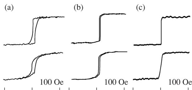
**Fig. 1.** Evolution of the form of the hysteresis loops of Co<sub>45</sub>Fe<sub>45</sub>Zr<sub>10</sub>/ $\alpha$ -Si nanostructures at a,  $y = 0.97$  nm; b,  $y = 1.7$  nm; c,  $y = 4.45$  nm. (Loops are measured in two mutually perpendicular directions).
