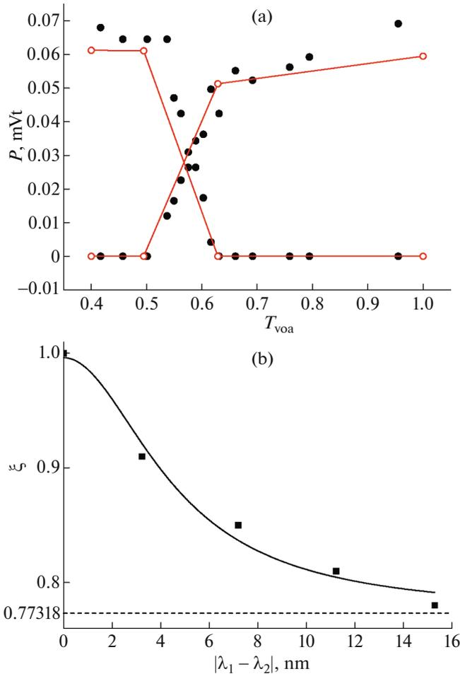
**Fig. 4.** The experimental (dotted curves) and theoretical (solid curves) dependences of the two-channel powers on the attenuator transmission of one of the channels. The match between the experimental and theoretical dependences is provided by the choice of the cross-saturation coefficient value  $\zeta$  (a). The dependence of the cross-saturation coefficient,  $\zeta$ , on the frequency spacing between the channels (b).
