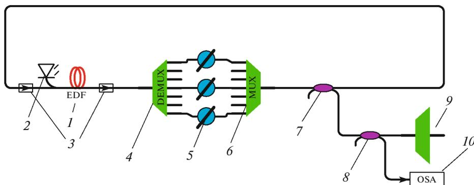
**Fig. 1.** The experimental device: an erbium-doped fiber (1), a diode pump laser (2), an optical insulator (3), multiplexers (4, 6, 9), a tunable attenuator (5), optical splitters (7, 8), and an optical spectrum analyzer (10).
