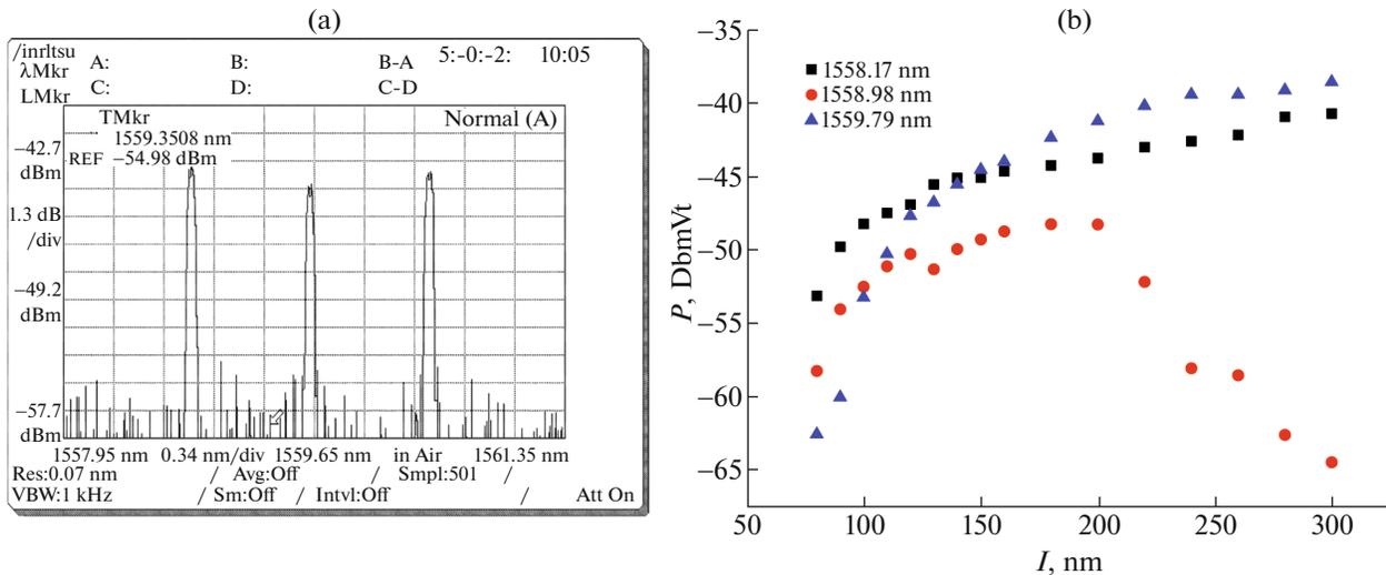
**Fig. 3.** The three-channel generation spectrum at a frequency spacing between the channels of 100 MHz (a) and the dependences of the channel output powers on the pump current (b).
