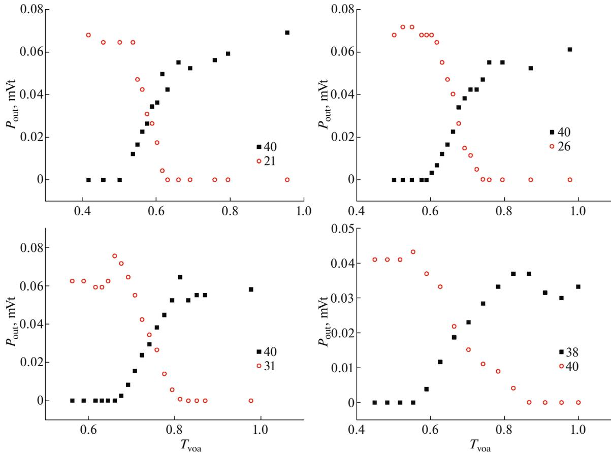
**Fig. 2.** The dependences of the powers of the channels on the losses in the controlled channel (black squares).  $T_{\text{voa}}$  is the attenuator transmission coefficient. The channel numbers are given in the legends.
