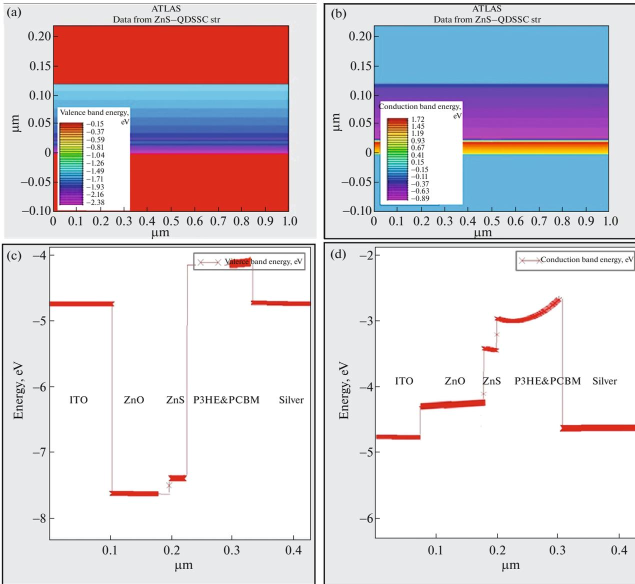
Fig. 5. (a), (c) The valence band energy, (b), (d) the conduction band energy diagrams of ZnS QDSSC layers.
