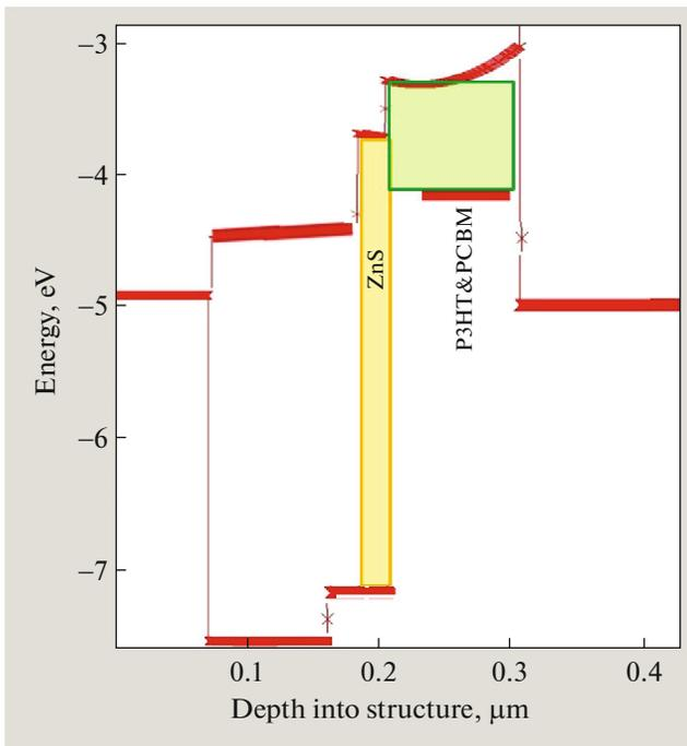
**Fig. 6.** Valence and conduction bands energies for active layers.
