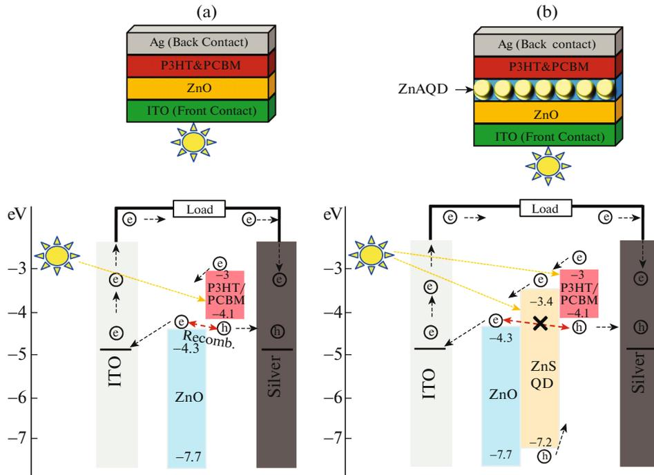
**Fig. 1.** Schematic diagram and energy level position of layers in (a) OPV, (b) ZnS QDSSC. The probable recombination is passivated with ZnS QD layer.
