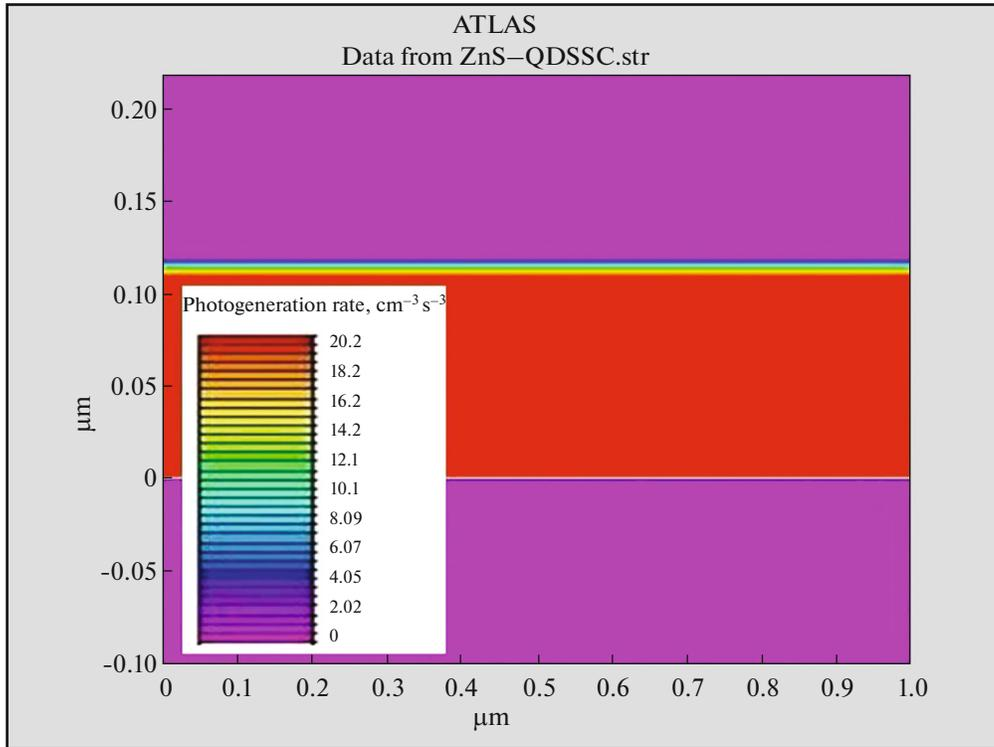
Fig. 4. Photo-generation rate obtained from simulation.
