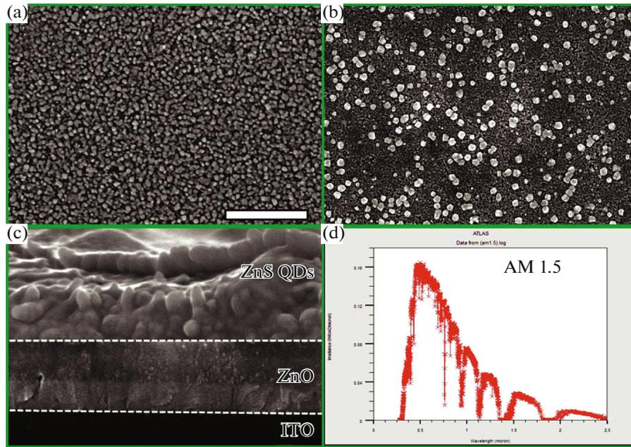
**Fig. 2.** SEM images of (a) ZnO film, (b) ZnS QD layer, (c) Cross sectional view of ITO/ZnO/ZnS QD layers, and (d) air mass spectrum 1.5 used to illuminate the model. Scale bar: 1  $\mu\text{m}$ .
