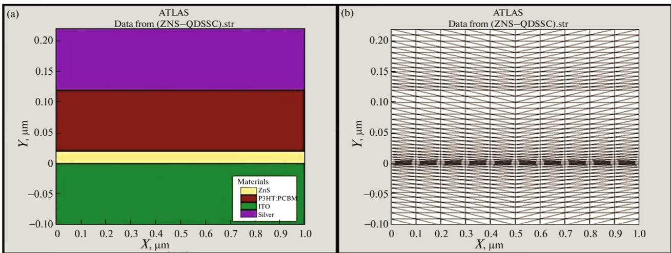
**Fig. 3.** (a) ZnS QDSSC structure, (b) 2D meshing of ZnS QDSSC.
