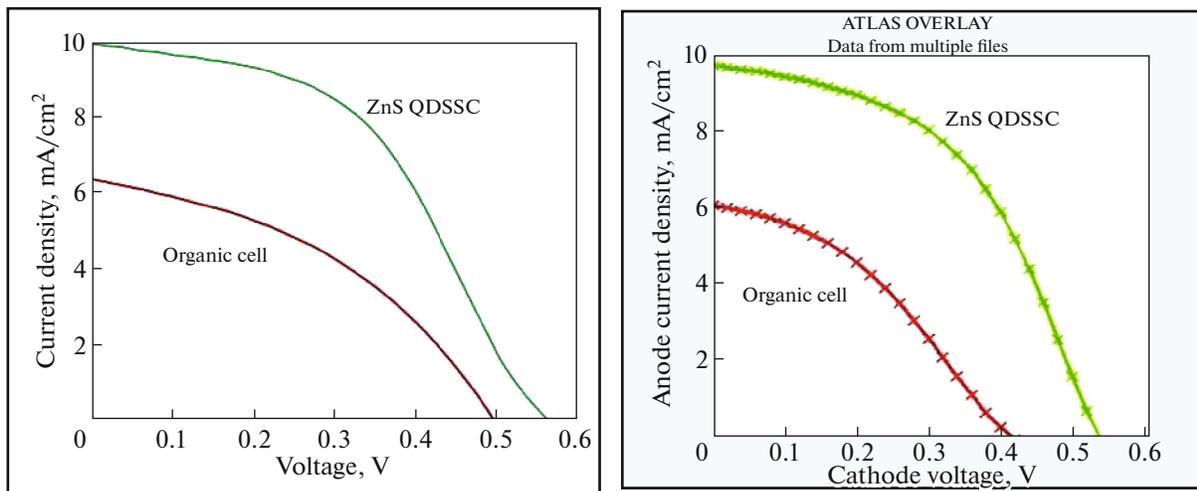
**Fig. 7.**  $J$ – $V$  curves of OPV and ZnS QDSSC obtained (a) experimentally, (b) from simulation.
