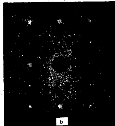
Fig. 2. Schematic of micro-electron diffraction pattern of the (110)_{\beta} plane (a); experimental micro-electron diffraction pattern of the Zr-Mo-Al alloy after 15 hr of tempering at 350^{\circ}\text{C} (b).
