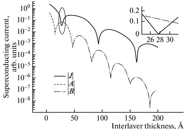
**Fig. 3.** Dependence of the critical current (solid line) and Harmonics  $A$  and  $B$  of current–phase relation on interlayer thickness (dashed and dashed–dotted lines, respectively). The region of the first minimum of the first harmonic (25–31  $\text{\AA}$ ) is shown in the insert. The dashed line on the insert shows the doubled  $B$  harmonic. The region where the quibit conditions satisfy: 27.7–30.5  $\text{\AA}$ ,  $T = 0.5 \text{ K}$ ,  $l = 28 \text{ \AA}$ .
