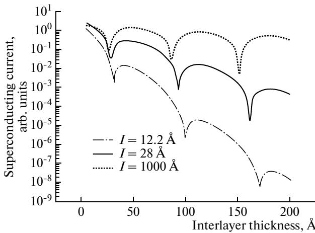
**Fig. 4.** Critical current as a function of interlayer thickness at different mean free paths  $l$ . The solid line ( $l = 28 \text{ \AA}$ ), the dashed-dotted line ( $l = 12.2 \text{ \AA}$ ), the dashed line ( $l = 1000 \text{ \AA}$ ). The region where the quibit conditions satisfy at  $l = 12.2 \text{ \AA}$ :  $30.55\text{--}31.1 \text{ \AA}$ ,  $T = 0.5 \text{ K}$ .
